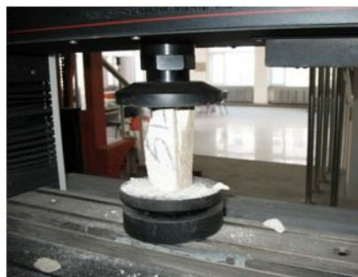
图 4 配比材料压缩试验 Fig.4 The compression test for simulated material
